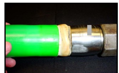
Flexible piping is bulging
