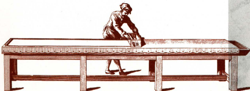
Jill Faulds and Lou Dolive are "running the sheet". The trough is filled with hot metal and run down the table, a granite slab covered with cloth. The metal runs out of a slit at the bottom to form a sheet. This chills quickly and is rolled up for storage. Various alloys of lead and tin are used for organ pipes, from almost pure lead to about 90% tin. Most organ people agree that the type of alloy has some effect on the sound. Though this point is sometimes hotly debated, it is almost never ignored.
