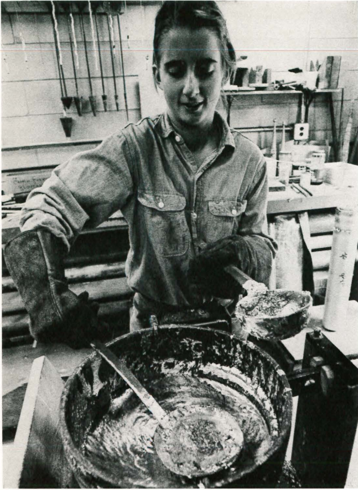
Jill Faulds skims the ladle. As the hot metal chills, the oxides which form on the top must be skimmed off. When the metal gets to the right temperature the pipe makers pour it into the trough and "run the sheet".
