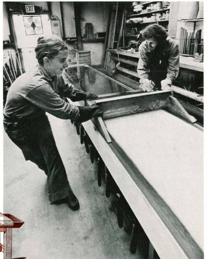
Jill Faulds and Lou Dolive are "running the sheet". The trough is filled with hot metal and run down the table, a granite slab covered with cloth. The metal runs out of a slit at the bottom to form a sheet. This chills quickly and is rolled up for storage. Various alloys of lead and tin are used for organ pipes, from almost pure lead to about 90% tin. Most organ people agree that the type of alloy has some effect on the sound. Though this point is sometimes hotly debated, it is almost never ignored.
