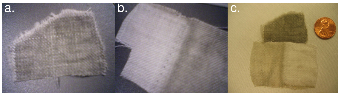
Figure 6. Samples of outer fabric from Apollo 12 LMP spacesuit. (a) Outer surface of T-164 Teflon ® outer abrasion fabric from left knee, (b) T-164 Teflon ® fabric swatch from left shoulder; lighter area was covered under U.S. flag patch. (c) Comparative size of swatches shown in (a) and (b).
