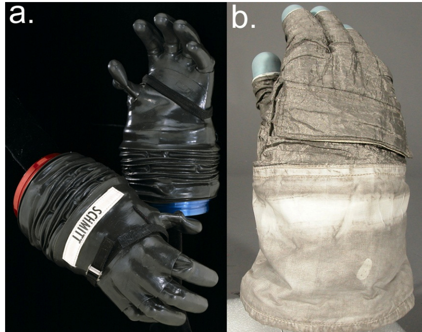
Figure 26. Examples of the two types of Apollo spacesuit pressure gloves.( a) Apollo 17 LMP IV pressure gloves, and (b) Apollo 17 LMP EV pressure glove. (Official Smithsonian images used by permission).
