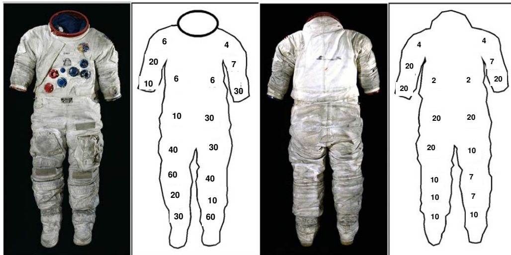
Figure 24. Concentration of Ti in units of \text{ppm} \times 10^2 measured by ED-XRF for tape-sampled location on front (left) and back (right) of Apollo 17 LMP ITMG (see Fig. 14).
