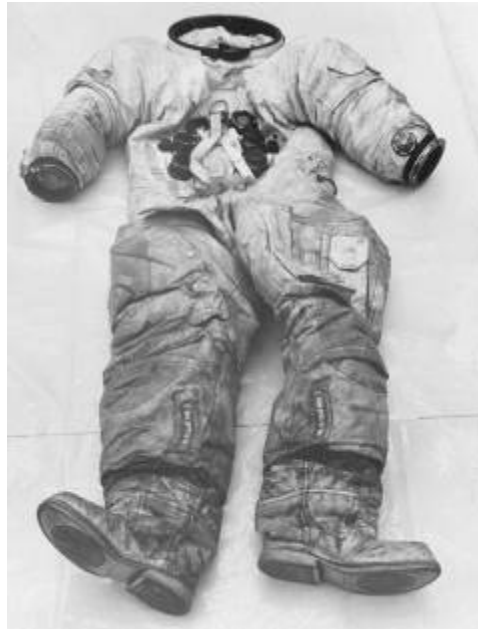
Figure 5. ITMG from model A7L spacesuit worn on the lunar surface by Apollo 12 LMP Alan Bean. Image originally appeared in NASA TR-169-001, prepared at the WSTF.
