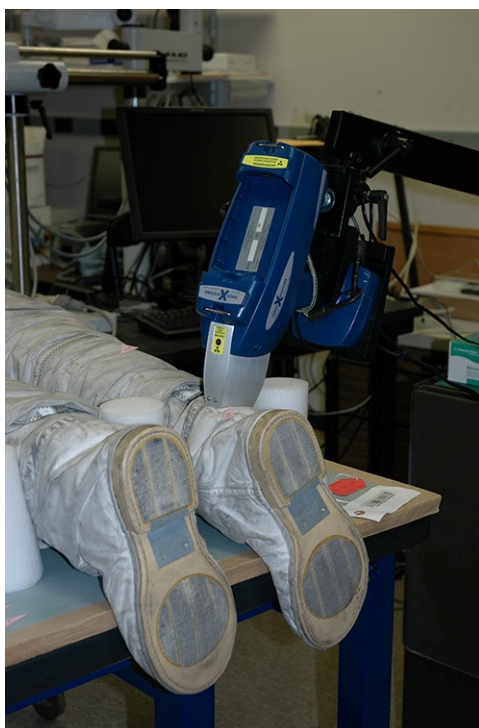
Figure 3. Innov-X Systems portable ED-XRF spectrometer (blue unit), which is held in a positioning tripod for chemical analysis of the outer fabric of the Apollo 17 spacesuit.
